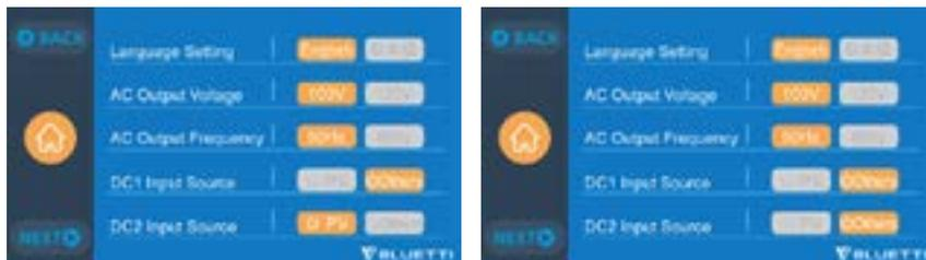
Method d: PV Parallel (PV parallel needs to be set in “Settings”)
